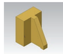
GB = Gusset Back: having a fin on one side that is not attached to the belt but rests on it and increases rigidity when the cleat is pushed in one direction
