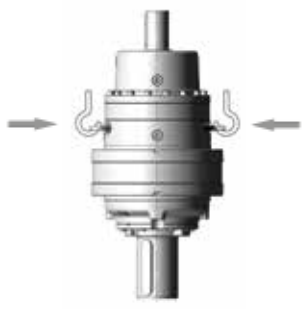
⊗ Lifting and handling incorrect
