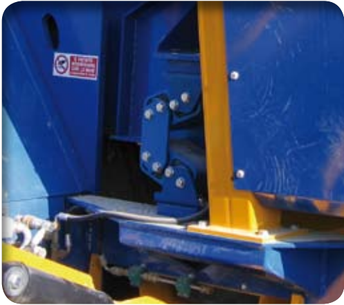
Suspensions of waist feeder to crusher
