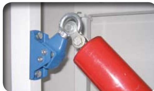
Protective suspension of belt transfer stations
