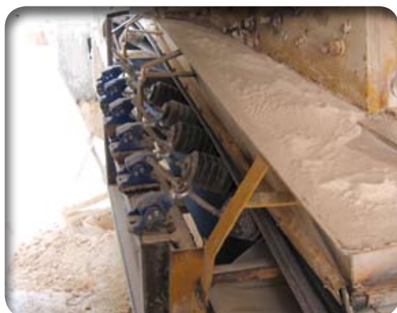
Protective suspension of belt transfer stations
