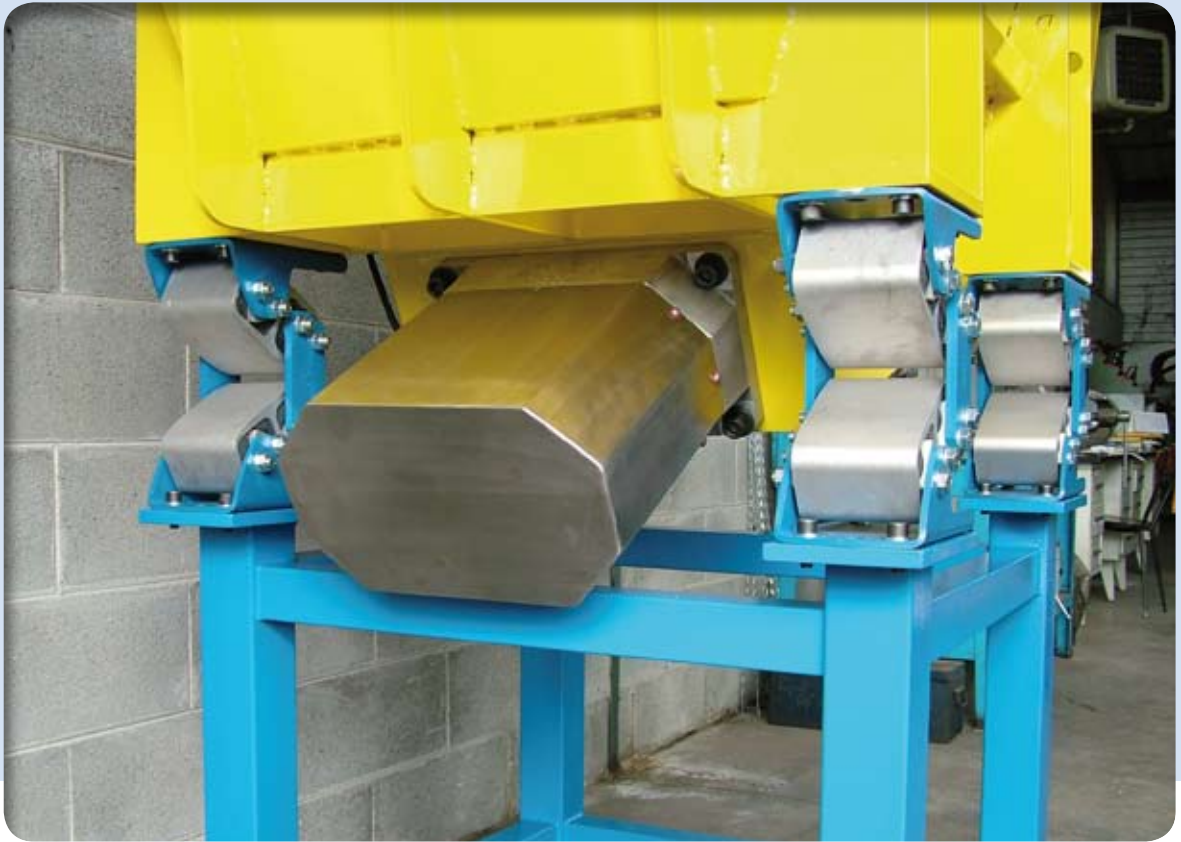
Elastic suspensions for electromagnetic excitation
