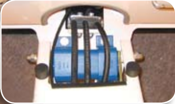
◀ Resilient handle mounting for vibrating compactors
