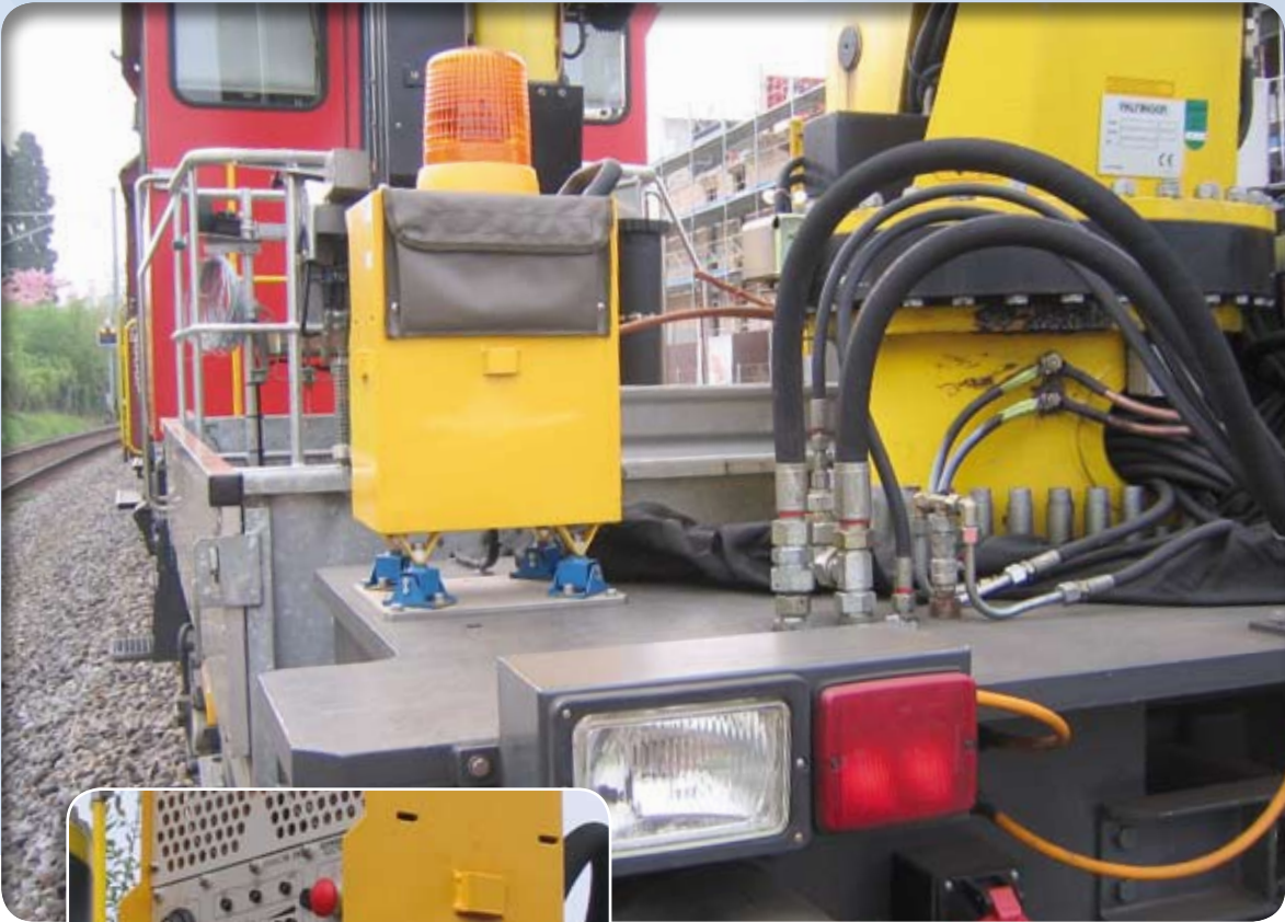
▲ Protective suspension of electronic device on track car
