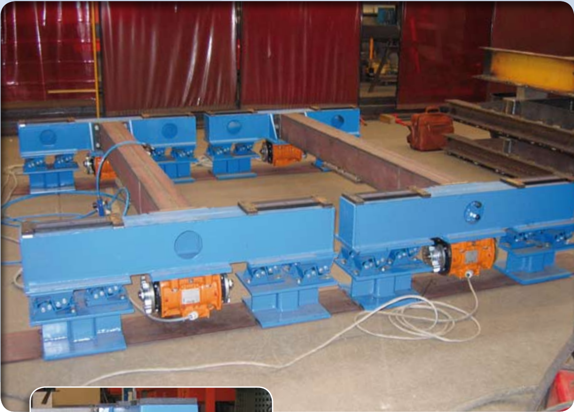
Resilient suspension of compactor for prefabricated concrete slabs
