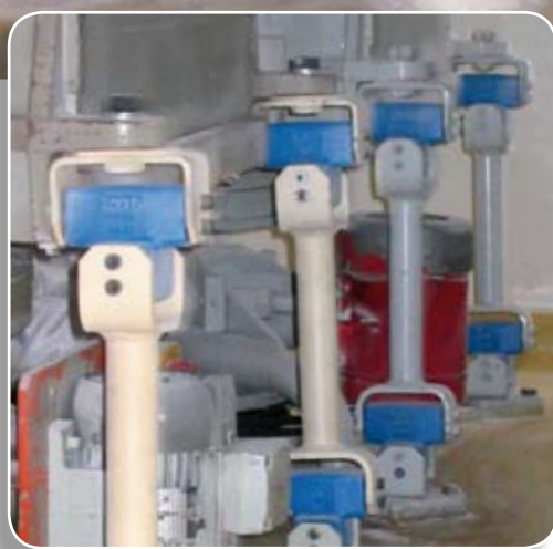
Universal joint suspensions for crank driven sifters
