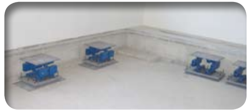
Protective suspension of mass-bed in laboratory
