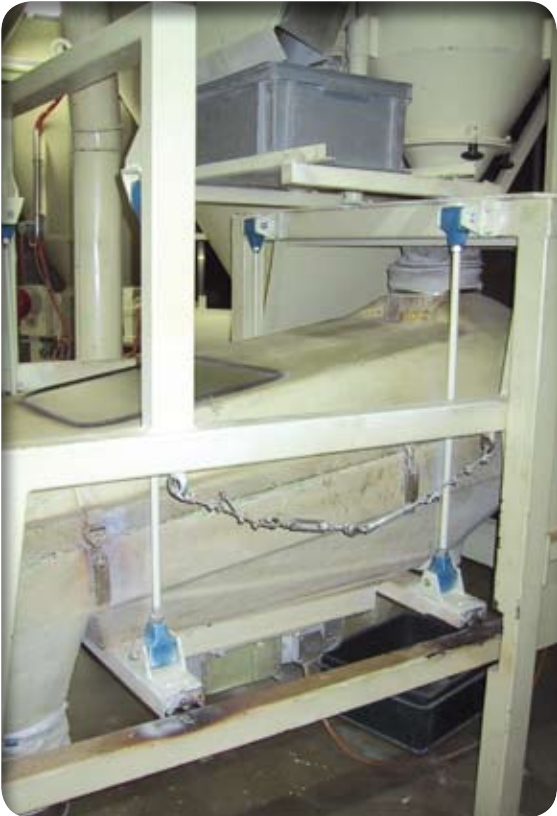
Universal joint suspensions for crank driven and free oscillating sifters
