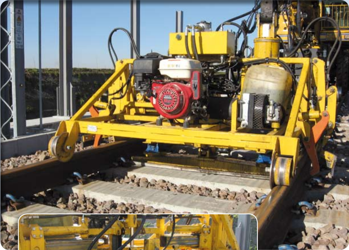
Cushioning suspension of railway-bed compactor
