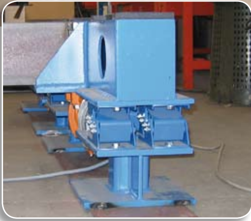
Resilient suspension of compactor for prefabricated concrete slabs
