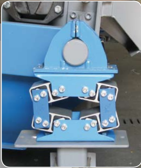
Suspensions of circular motion screen pivot system
