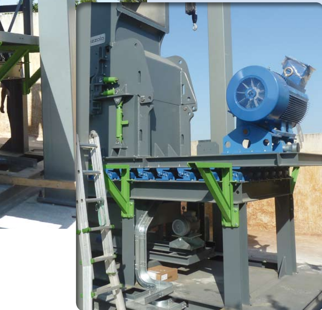
Crusher protective suspensions
