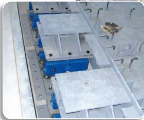
Protective suspension of mass-bed in laboratory
