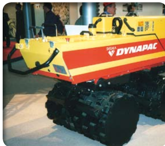
Resilient handle mounting for vibrating compactors
