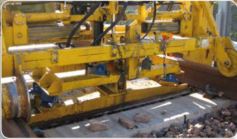
Cushioning suspension of railway-bed compactor
