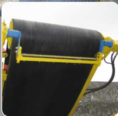
Elastic scraper suspensions for continuous belt cleaning
