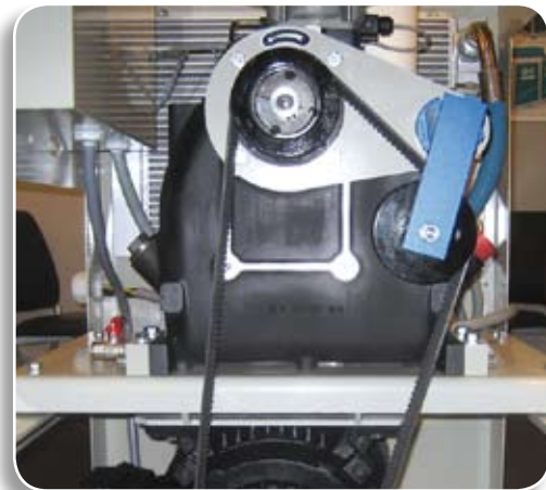
Elastic belt tensioning devices between drive motor and compressor
