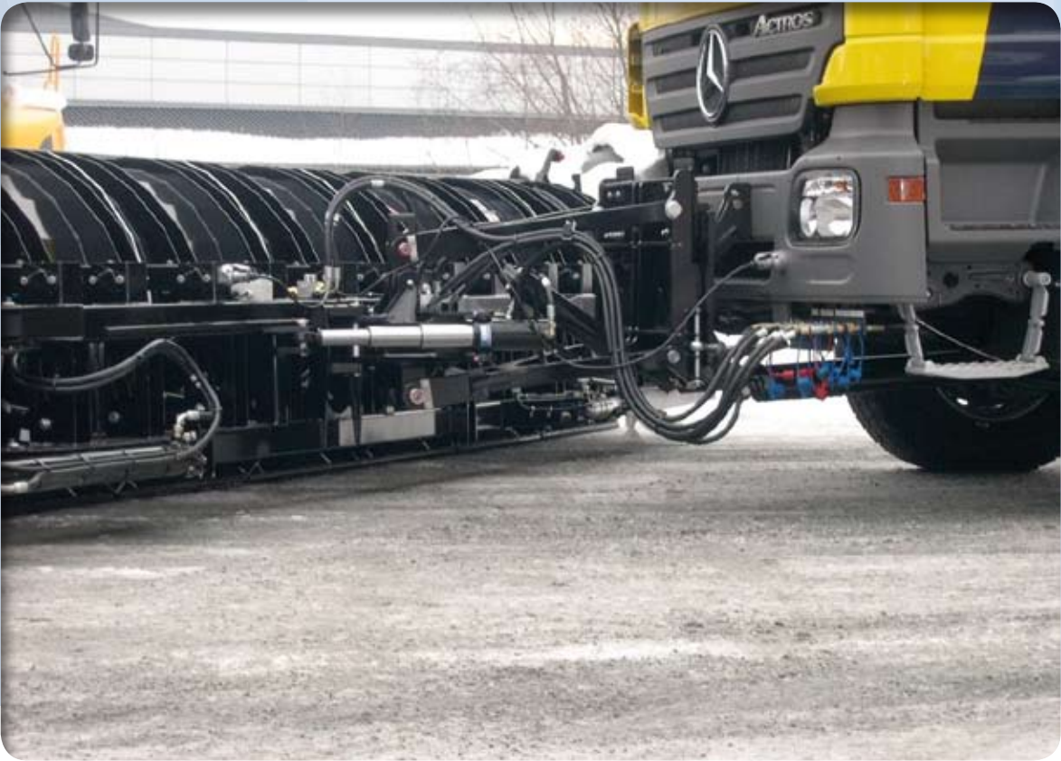
Elastic parallelogram suspensions of plough blades with double rockers
