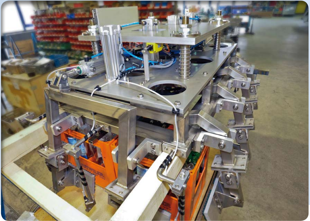
Gripper mechanism for beverage industry
