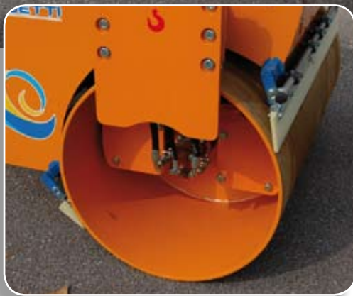
Elastic scraper suspensions for roll cleaning
