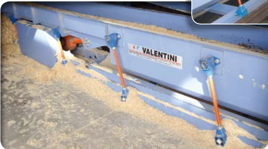
Rocker suspensions for conveyor troughs
