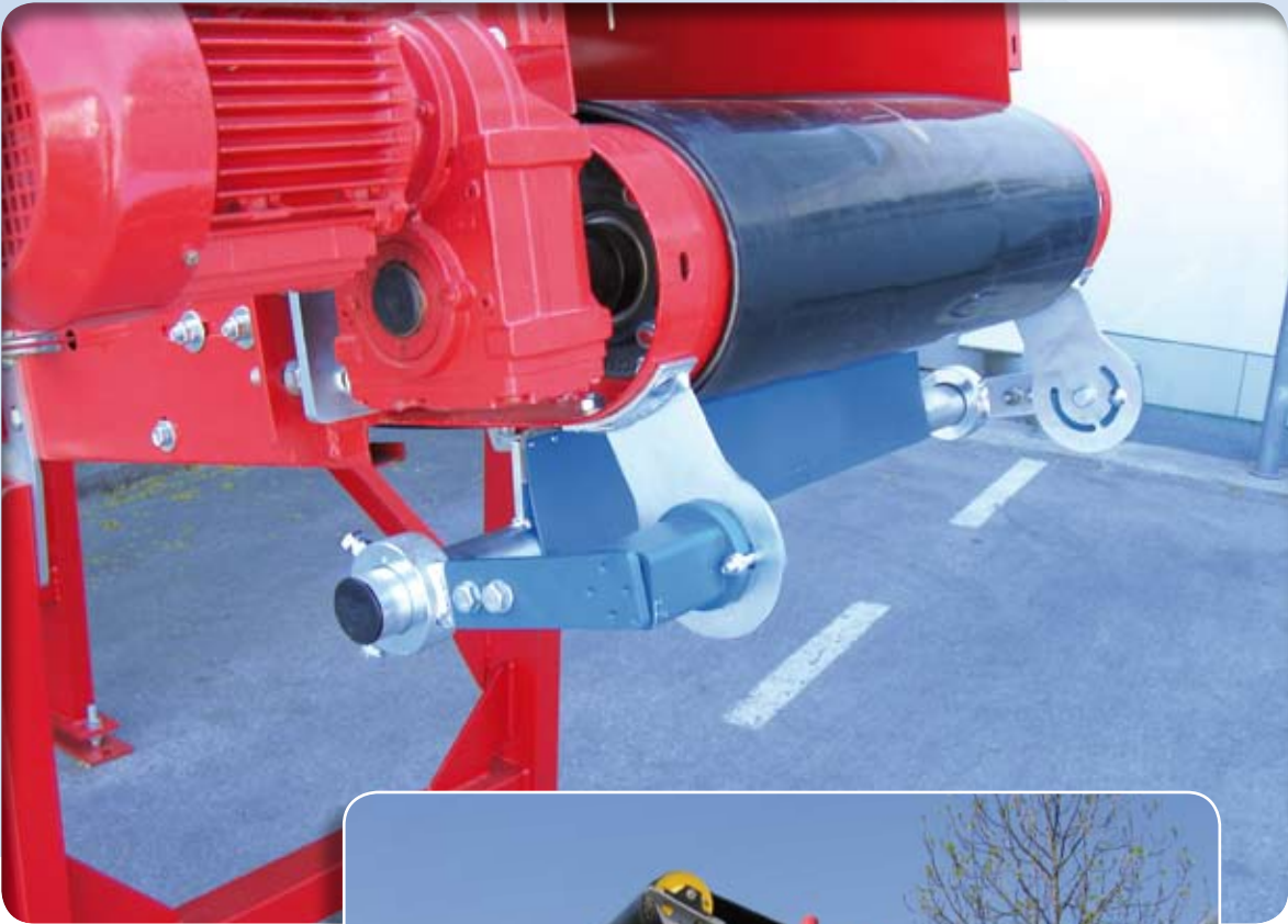
Elastic scraper suspensions for continuous belt cleaning
