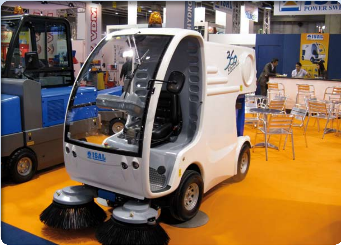
▲ Elastic suspension of rotary brush
