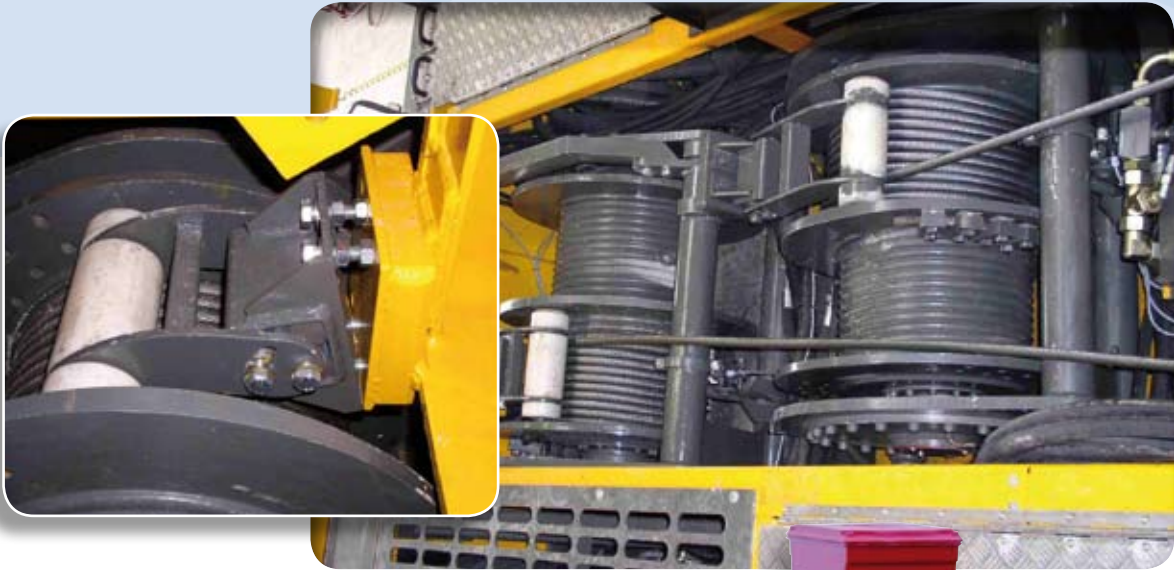
Guide roller suspensions for controlled cable reeling on winch drum
