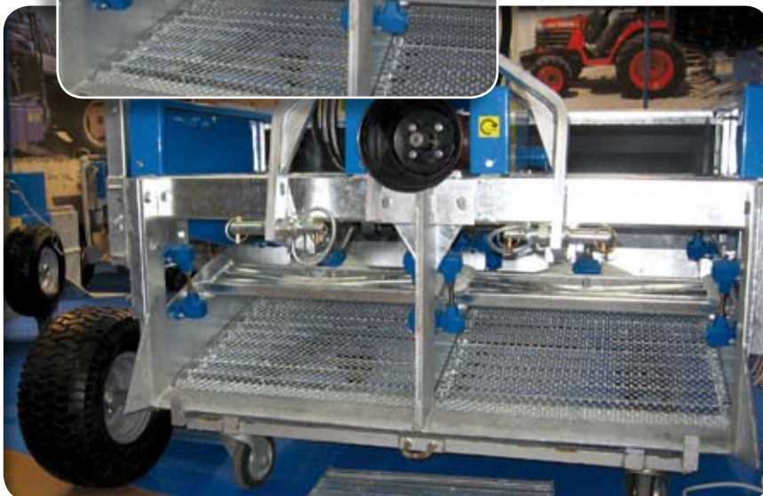
Elastic rocker suspensions for sand sifting screens
