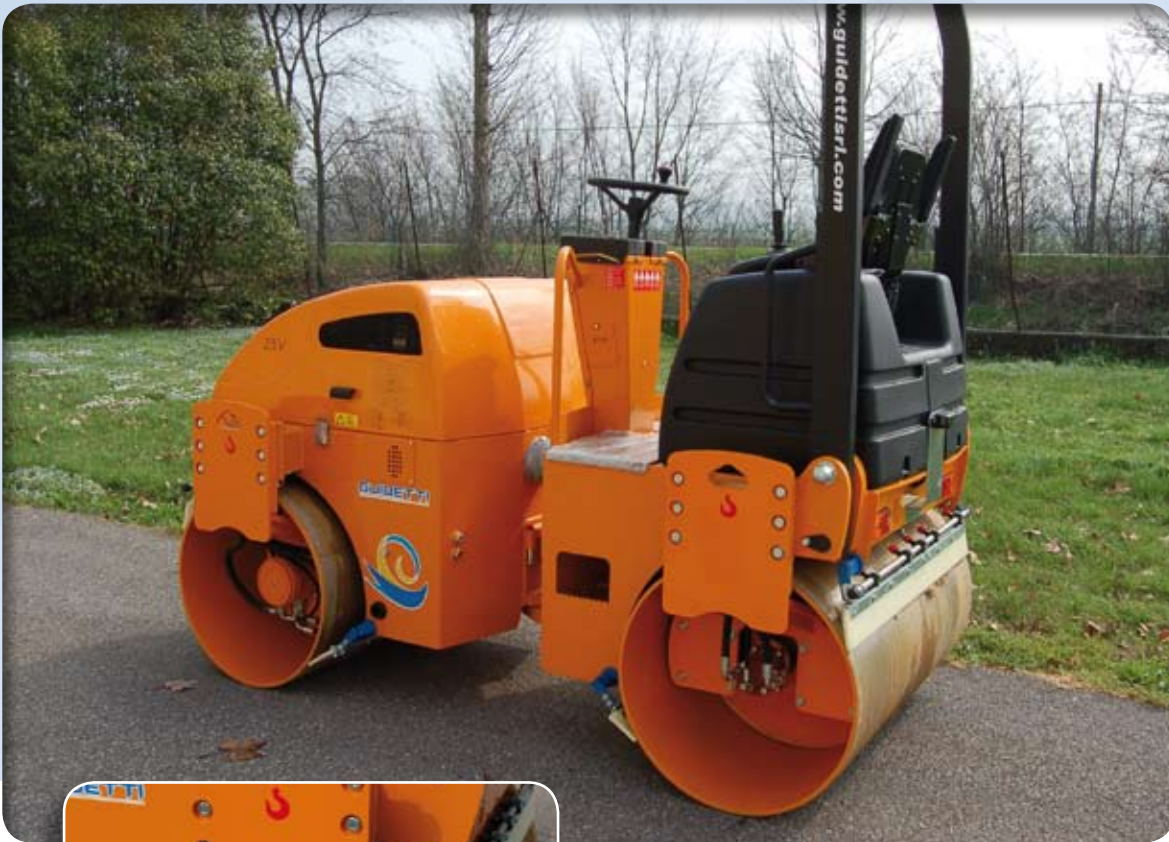
Elastic scraper suspensions for roll cleaning
