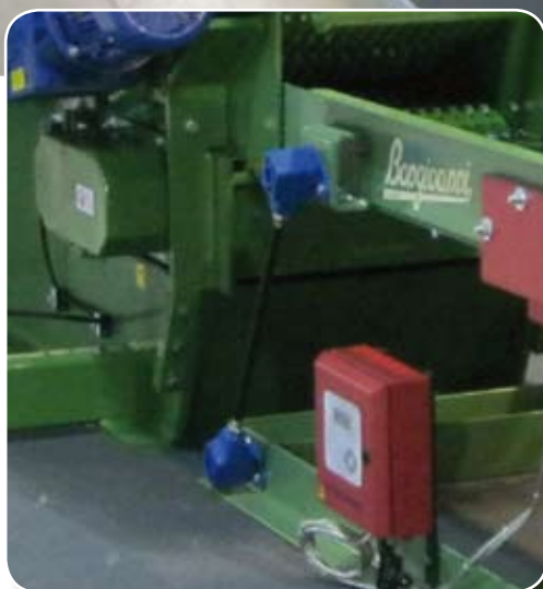
Rocker suspensions for conveyor troughs
