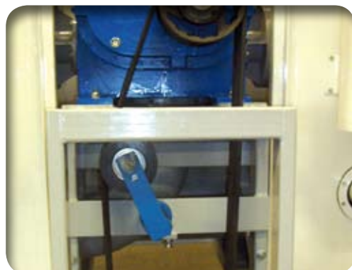
Elastic belt tensioning devices between drive motor and compressor
