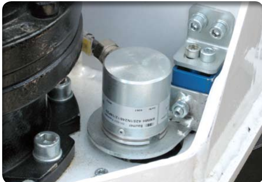
Elastic torque bracket for hydraulic motor
