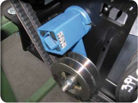
Elastic belt tensioning devices
