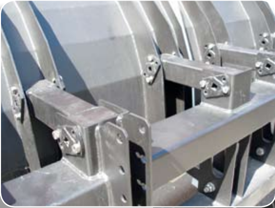
Elastic parallelogram suspensions of plough blades with double rockers
