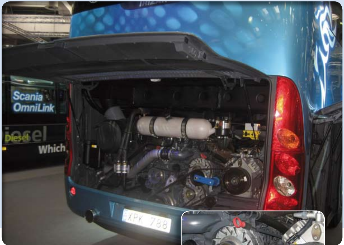
Belt tensioners for drive between diesel engine and cooling compressor
