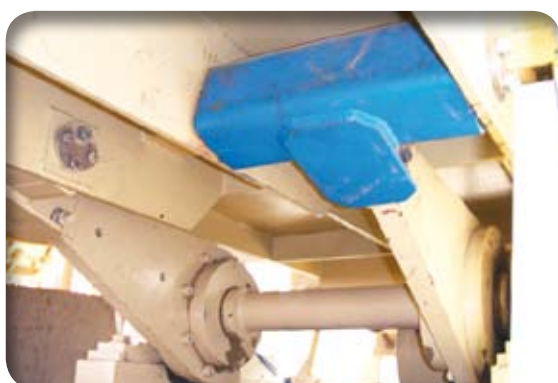
Elastic drive heads for crank driven troughs
