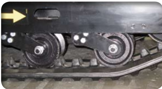
Elastic guide-wheel suspension for crawler mounted vehicles
