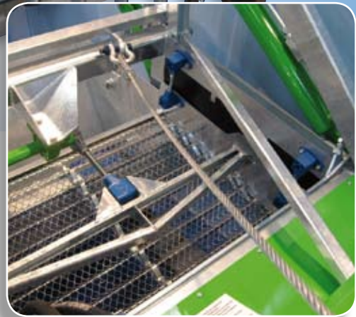
Elastic rocker suspensions for sand sifting screens
