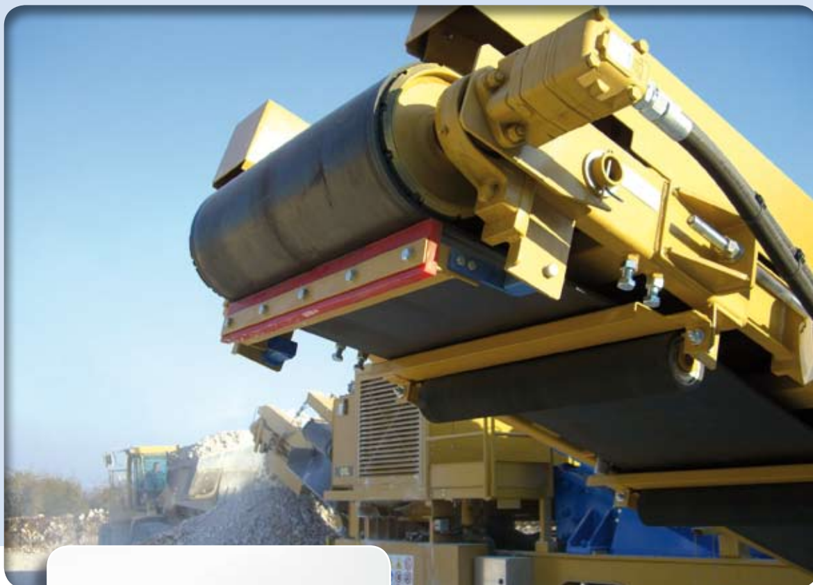
Elastic scraper suspensions for continuous belt cleaning
