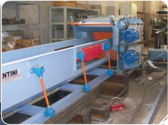
Rocker suspensions for conveyor troughs
