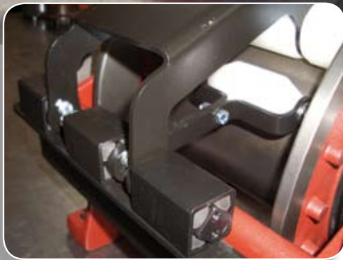
Guide roller suspensions for controlled cable reeling on winch drum
