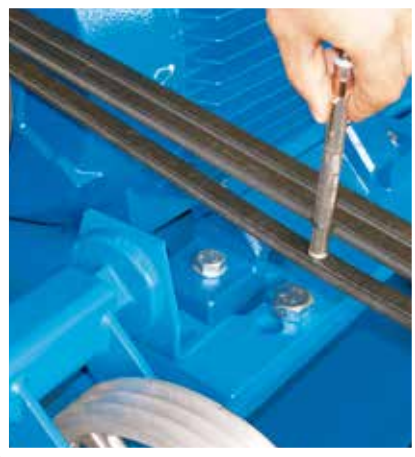
Spring scale tester from Gates
