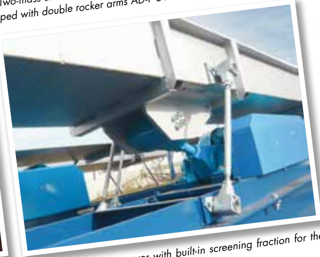
Two-mass "natural frequency" shaker conveyor equipped with double rocker arms made out in light metal casting
